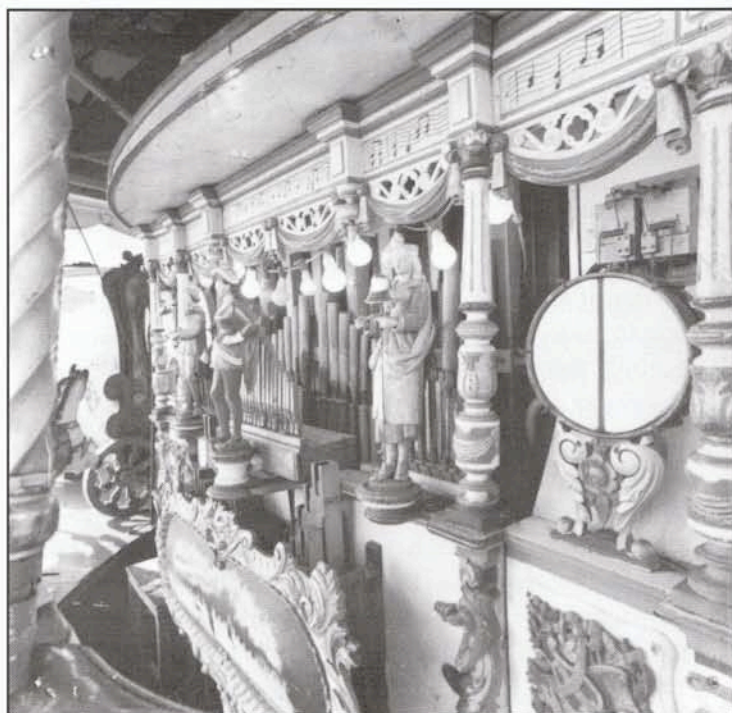
Figure 4. The Gavioli mounted in a smaller galloper post-conversion to the 89 VB scale, probably in the 1960s. The violin pipes are removed from the organ in this photo. Photo courtesy of Rosie Sreeton Armitage.
