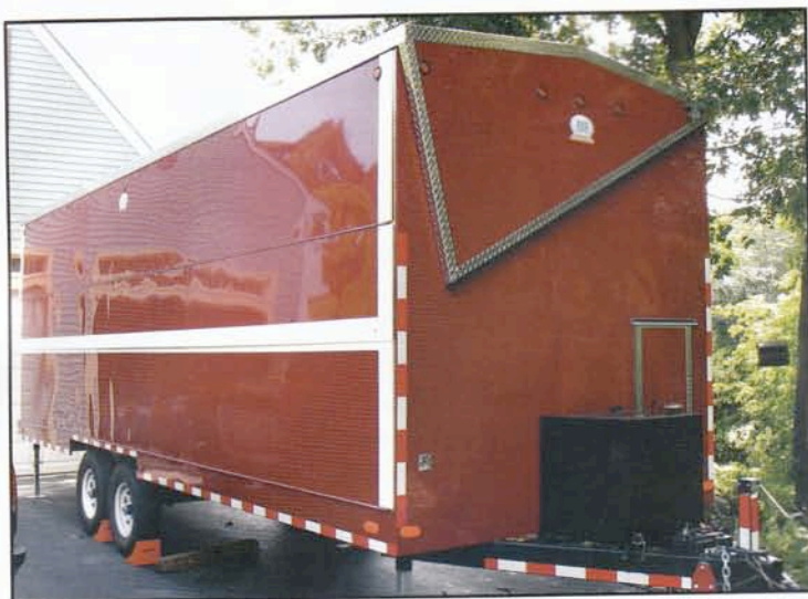
Figure 9. The display trailer is ready to travel. The trailer is 24 ft long (without tongue), 11'4" tall when traveling and 8' wide. It carries a 5500 watt diesel generator and sufficient fuel to run for 100 hours. Opening the trailer for display can be done by a single person.
